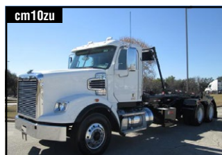
cm10zu 2023 FREIGHTLINER CORONADO 122 SD Detroit, DD13, 450 HP, Allison RDS automatic, 262" WB, 20k FA, 46k RA, 69,834 miles, Stk# 280778 . . . . . $199,995
